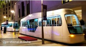
Compact example 2: TiG/m MRV-3 3 x 100 passenger vehicles operated by one 'driver' using semi-autonomous control
