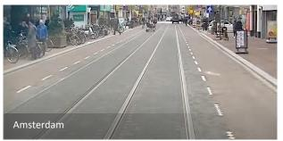
Shared Trambahn: Note, the broken white lines indicate that traffic in the right-hand lane including cyclists give way to trams
