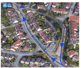
At the Bath Rd/Eagle Rd junction the double track would split into a single track running south on Bath Rd and a single track running north along Eagle Rd.
